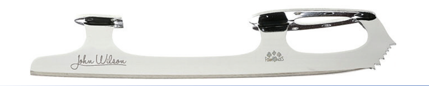
Four Aces - Traditional steel blade with straight cut picks, parallel siding and a 7 ft rocker. 7/16 radius of hollow.
